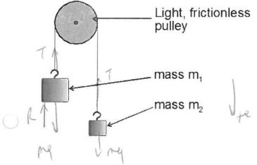
The diagram to the left shows a pulley system close to the ground. The mass of  $m_1$  is 7.58kg and the mass of  $m_2$  is 3.45kg.
