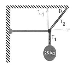
The diagram on the left shows a heavy chandelier suspended from a wall and ceiling.
