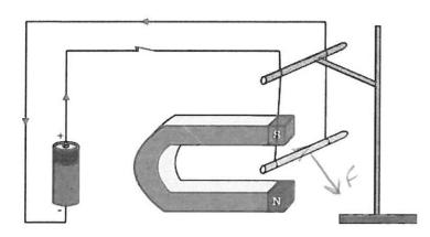
The diagram on the left shows a metal rod carrying a current of 0.560A, in a uniform magnetic field of 0.0540T. The uniform field extends along 13.5cm of the metal rod. The wooden retort stand on the right of the diagram has a horizontal wooden bar designed to hold the wires away from the magnet.
