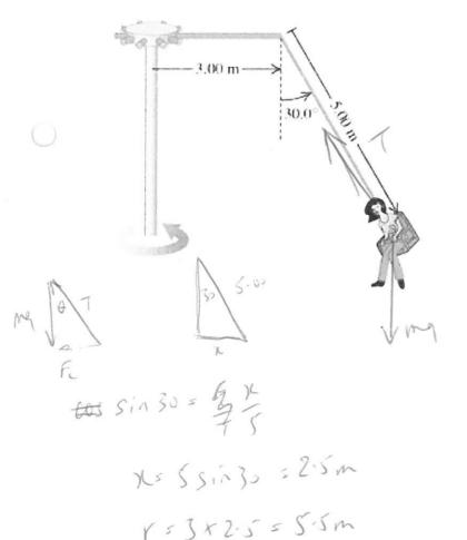
The diagram to the left represents a show ground ride that revolves at 5.00rpm.
