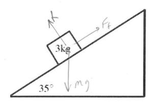
The diagram on the left shows a box of mass 3.00kg sliding down a ramp inclined at 35.00 to the horizontal, against a
