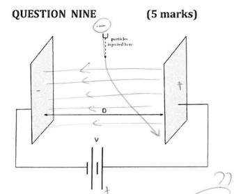
The diagram on the left shows a pair of metal plates separated by a distance, D, which is 14.5cm. The voltage applied across the plates is 245V, and the field established between the plates is uniform.
